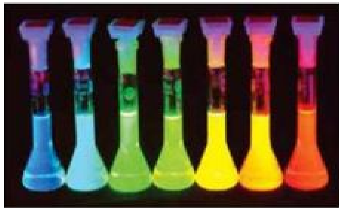
Fig.2 Variation in fluorescence with change in size of CdSe
