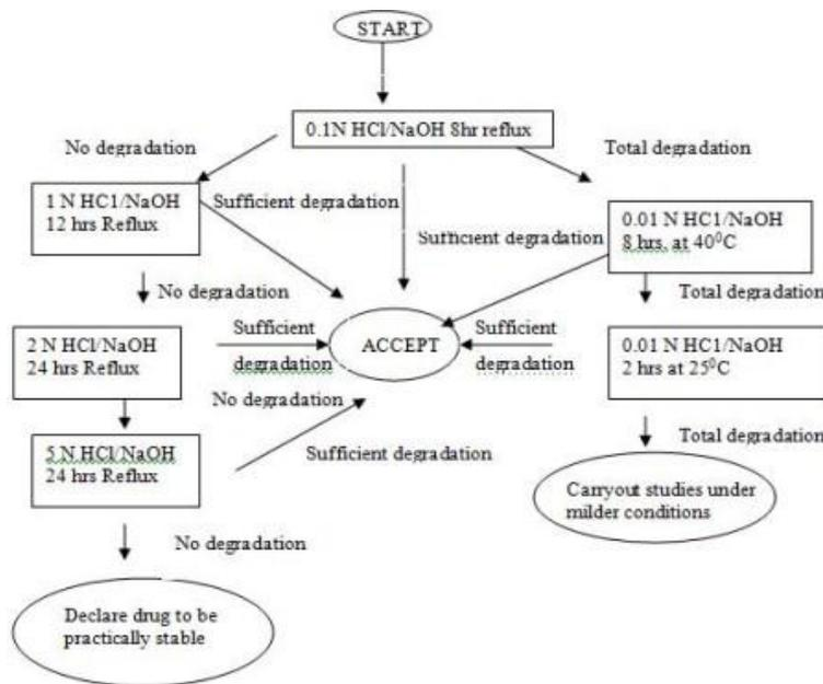
Figure 2: Flow chart of acid/alkali induced hydrolysis
