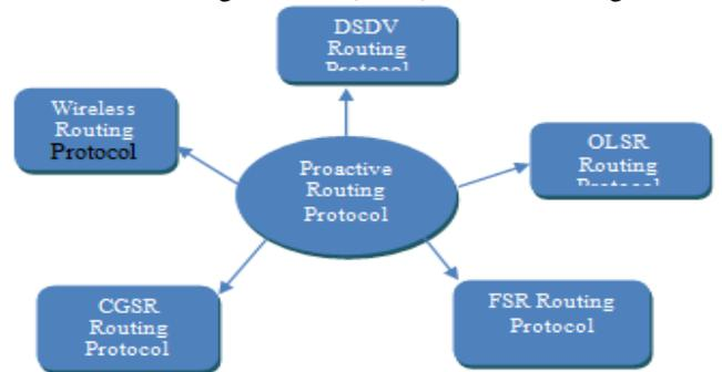
Figure 3 (Table Driven Routing Protocol)
