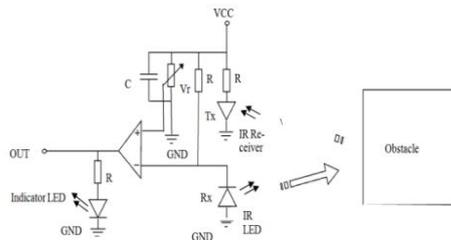
Figure1: The IR Sensor Schematic
