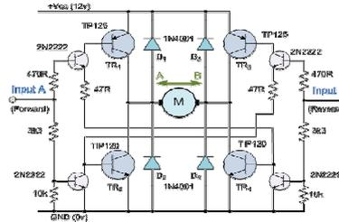
Figure6: H-bridge circuit diagram
