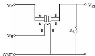
Figure2: This is the basic Circuit of GAS Sensor
