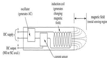
Figure4: Inductive Sensor Schematic
