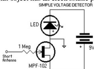
Figure3: The Discharge Sensor Schematic
