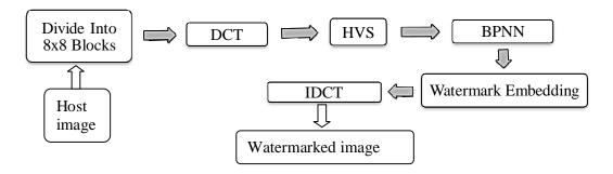
Figure 2: Watermark Embedding Block diagram
