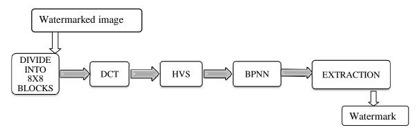
Figure 3: Watermark Extraction Block Diagram
