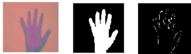
Figure 3.6: 1 shows YCbCr space image, 2 shows binary image, 3 shows canny edge detector image
