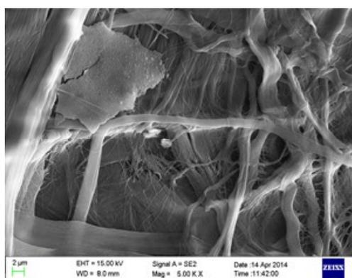
**Figure 1.2.** SEM image of a fractured section of a fish (*Puntius conchonius*) scale showing sliding of the collagen structure and pulling out and breakage of individual collagen fibers.
