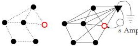
Fig. 2. A graph describing a sensor network  $G$  (left), and the associated fictitious electrical network  $G_{elec}$  (right).  $S$  Amp current is injected into the electrical network through the “source node” (unfilled circle), and extracted through the “ground” node (filled triangle). The line segments in the electrical network are  $1\Omega$  resistors.
