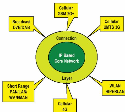
Fig 1: Seamless Connectivity of Communication Networks
