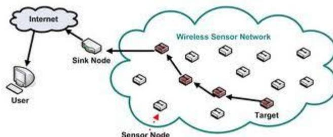
Fig.1. Wireless Sensor Network Diagram
