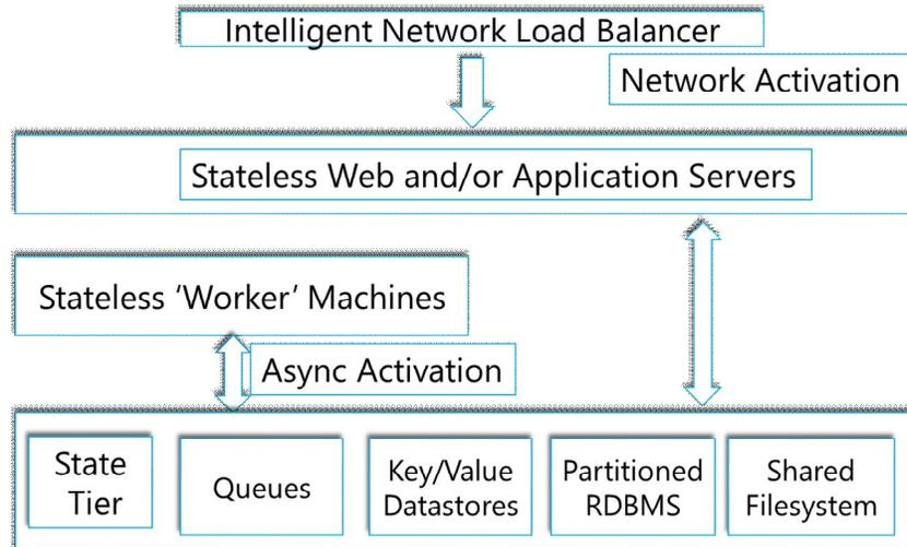
Fig. 15 Inbound Connectivity with Load Balancer
