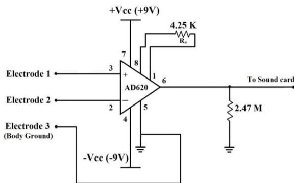
Fig.1 Circuit Diagram for sEMG sensor
