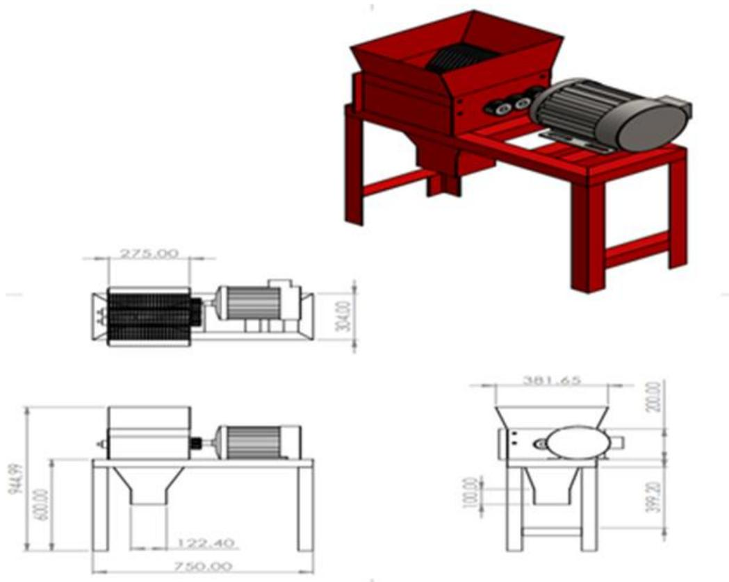
Figure 2. Exploded views of the shredding machine.
