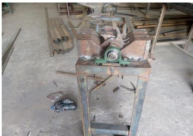
**Plate 2.** Shredder blade and shaft assembly.
