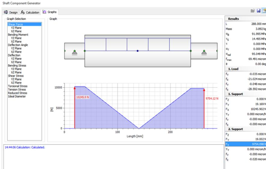
**Determination of shaft diameter:** The shaft diameter was estimated using equation 2. The basis considered were the maximum bending moment, torsion moment, shear stress, and diameter of the shaft.
