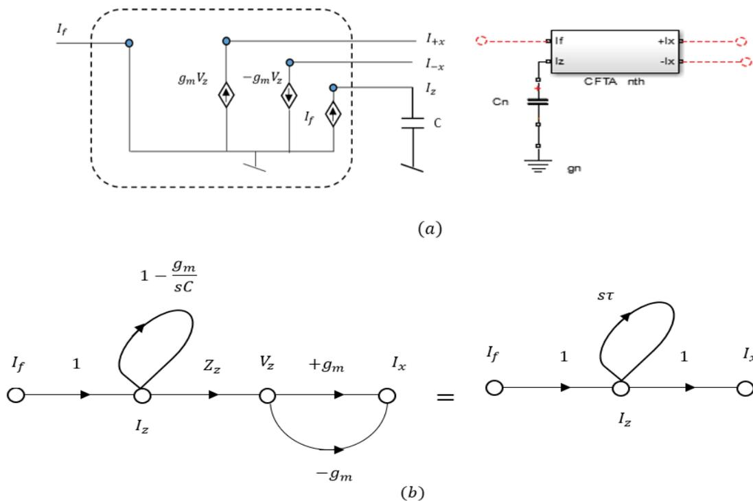
**Figure 6.** Sub-graphs and their corresponding Active-C sub-circuits involving CFTAs.
