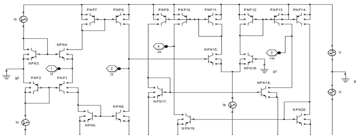
**Figure 18.** Bipolar implementation of the CFTA used for simulations.
