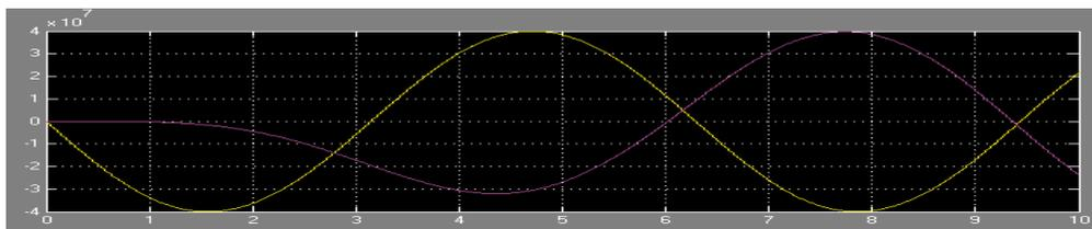
**Figure 23.** time domain response of proposed fourth-order all-pole low pass filter with respect to sinusoidal current output/input signal.
