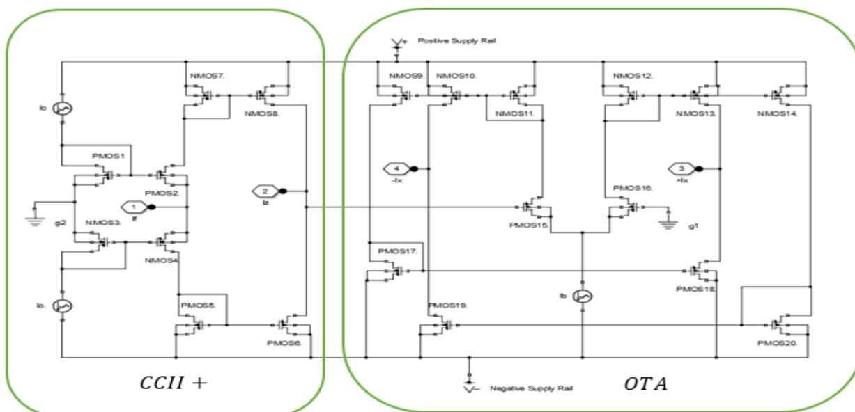
Figure 2. CMOS realization of the CFTA.
