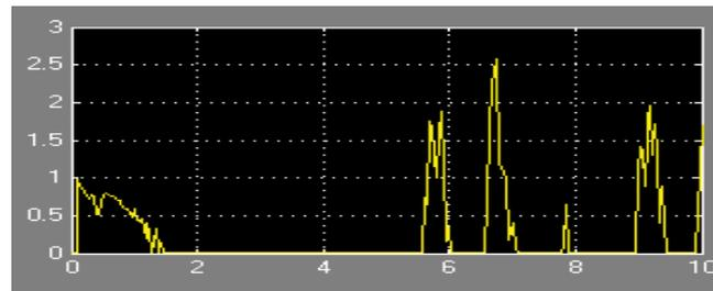
Figure 25. The THDs of the proposed fifth-order all-pole low pass filter.
