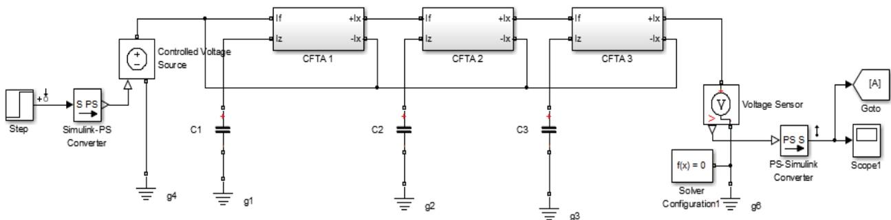
Figure 11. Model for third-order low-pass transfer function.
