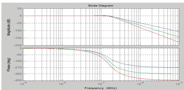
**Figure 21.** Gain and phase responses of the third, fourth and fifth-order all-pole low pass filter.
