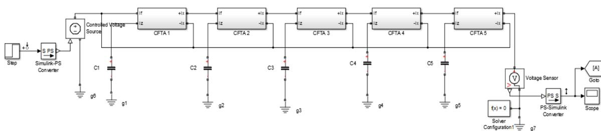
Figure 17. Model for the fifth-order low-pass transfer function.
