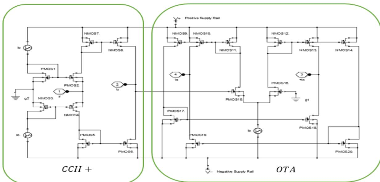
Figure 2. CMOS realization of the CFTA.
