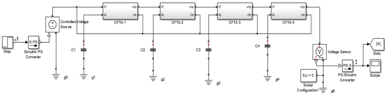
Figure 14. Model for the fourth-order low-pass transfer function.
