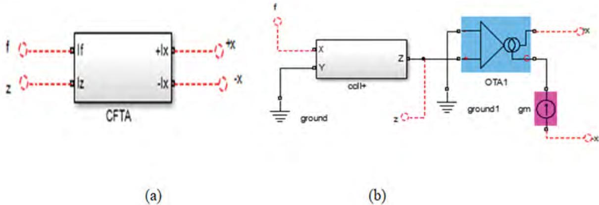
**Figure 3.** CFTA realization (a): block diagram implementation; (b): Implementation of the CFTA using CCII and OTA.
