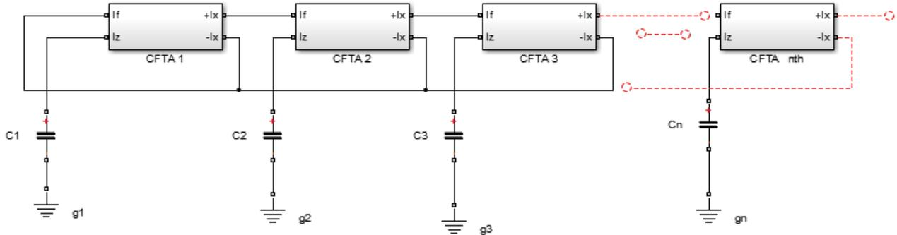
**Figure 7.** CFTA-based realization of the  $n$ -order current-mode low-pass filter, corresponding to the SFG given in **Figure 6**.
