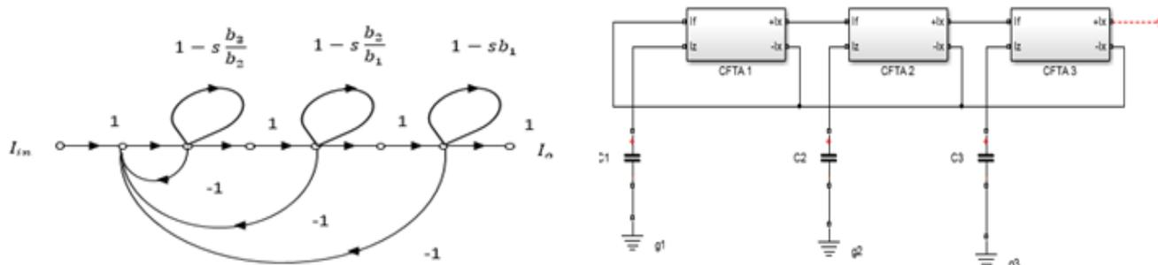
**Figure 9.** Third-order low-pass transfer function of equation (4): (a): signal flow graph representation; (b): circuit realization.
