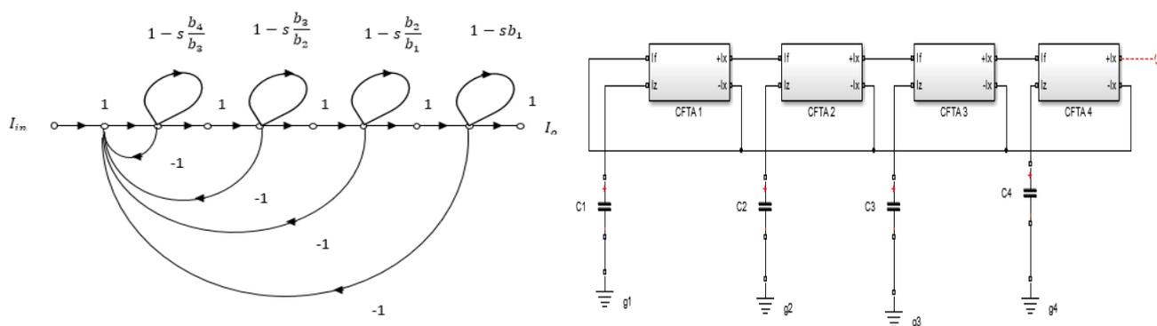
**Figure 12.** Fourth-order low-pass transfer function of equation (6), (a): signal flow graph representation; (b): circuit realization.
