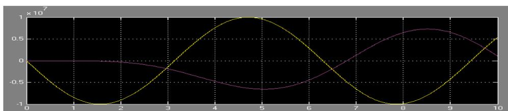
**Figure 24.** Time-domain response of proposed fifth-order all-pole low pass filter with respect to sinusoidal current output/input signal.
