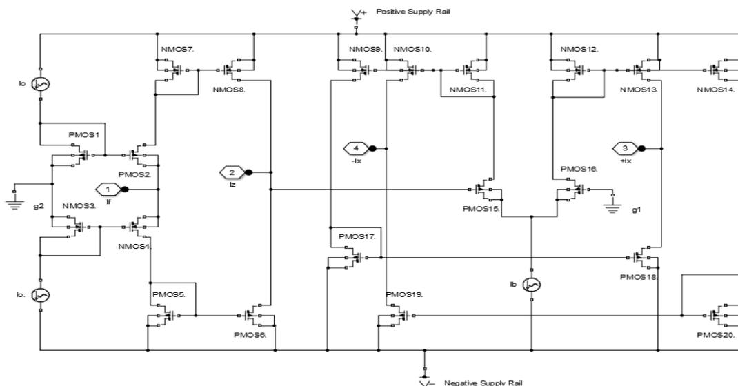
**Figure 20.** Simulated third, fourth and fifth-order all-pole low pass circuits.
