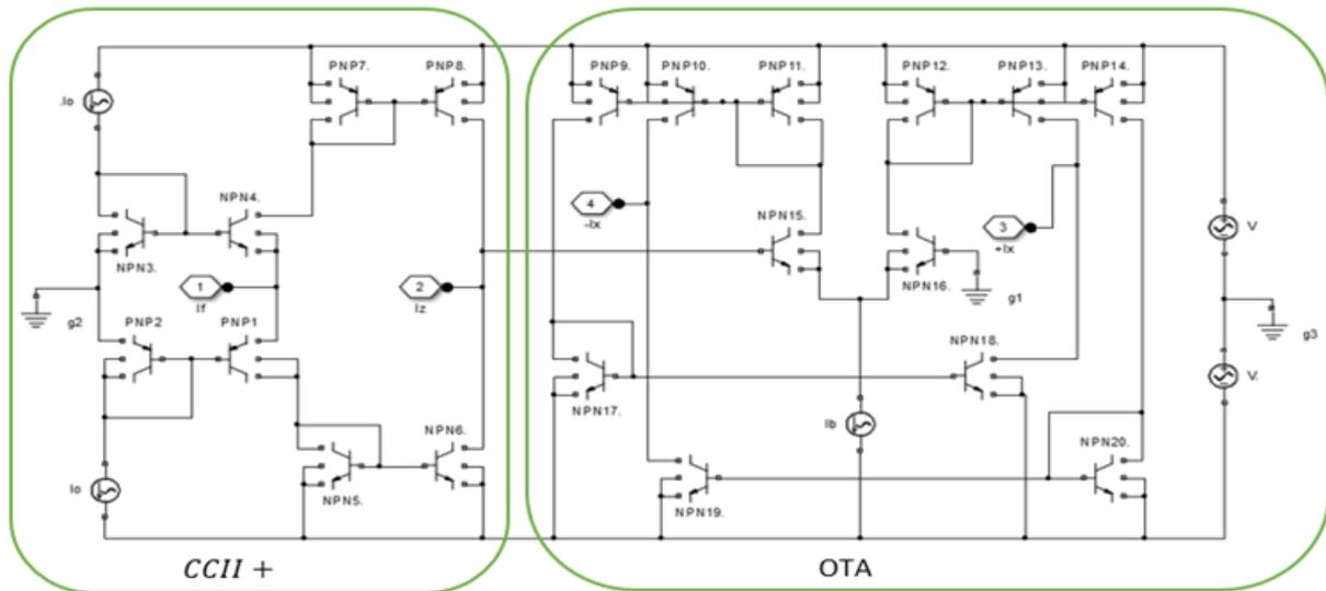
Figure 1. Bipolar realization of the CFTA.
