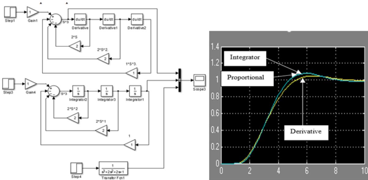
Figure 10. The state-space representation of the transfer function.
