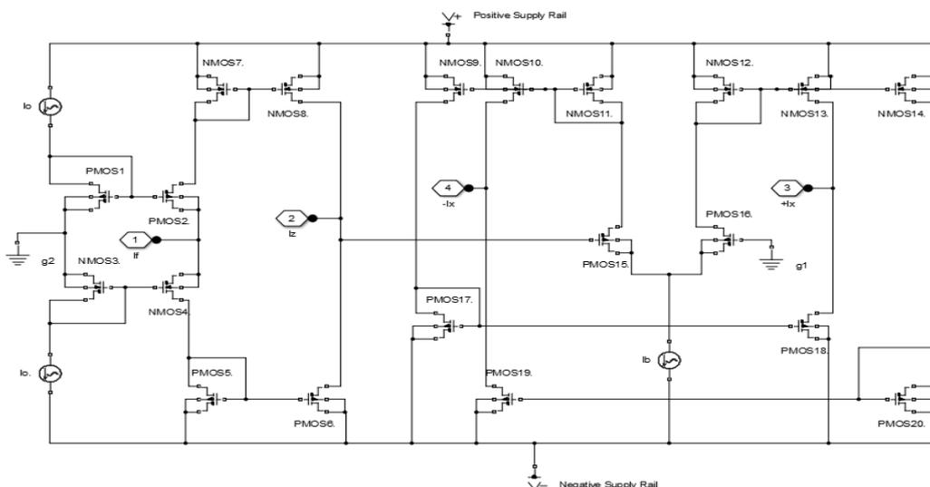
**Figure 19.** CMOS implementation of the CFTA used for simulations.
