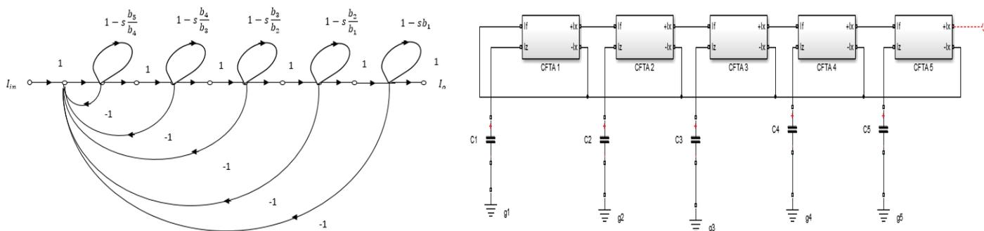
**Figure 15.** Fifth-order low-pass transfer function of equation (7), (a): signal flow graph representation; (b): circuit realization.
