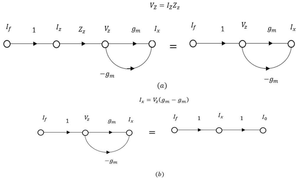
**Figure 5.** Signal flow graphs (a): cascade transformation and; (b): parallel transformation.
