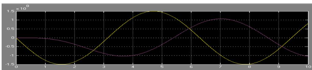
**Figure 22.** Time-domain response of proposed third-order all-pole low pass filter with respect to sinusoidal current output/input signal.
