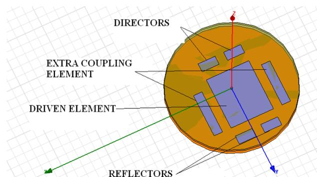
Fig3. Proposed yagi microstrip antenna
