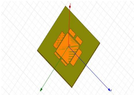
Fig7 Rectangular yagi patch antenna
