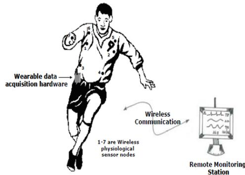
Fig1. Overall architecture of the wireless sensor network based wearable physiological monitoring system.
