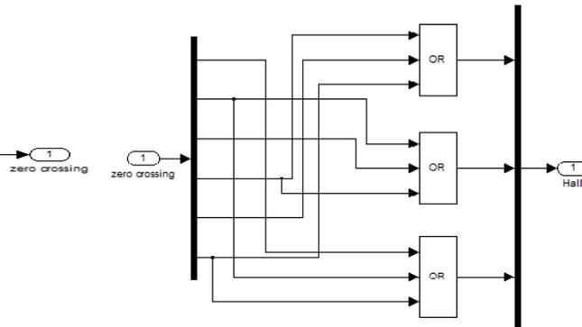
Fig 6 ZCD Decoding model
