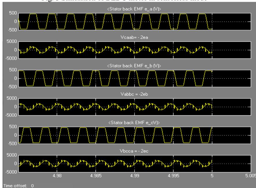
Fig. 4 Back EMF and corresponding line voltage difference waveforms
