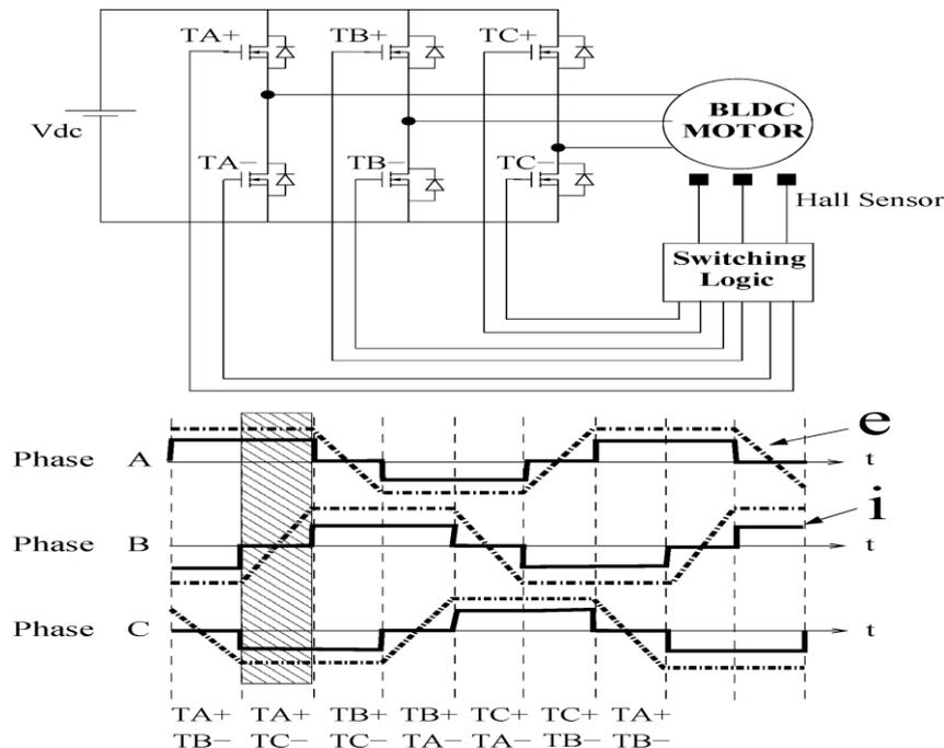
Fig.1. BLDC motor drive along with typical phase current and back EMF[8]
