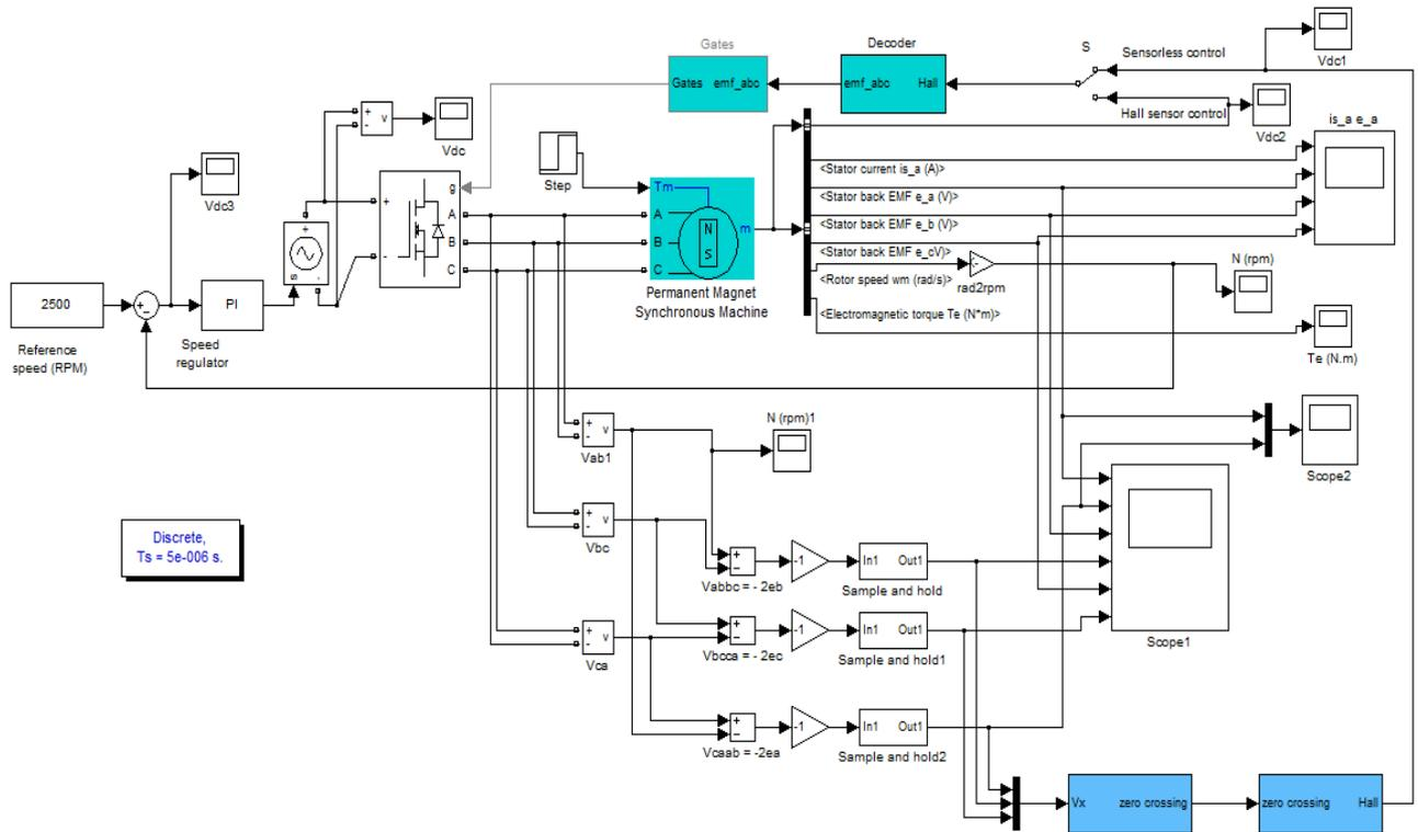
Fig. 3 Simulation of BLDC motor in sensorless mode
