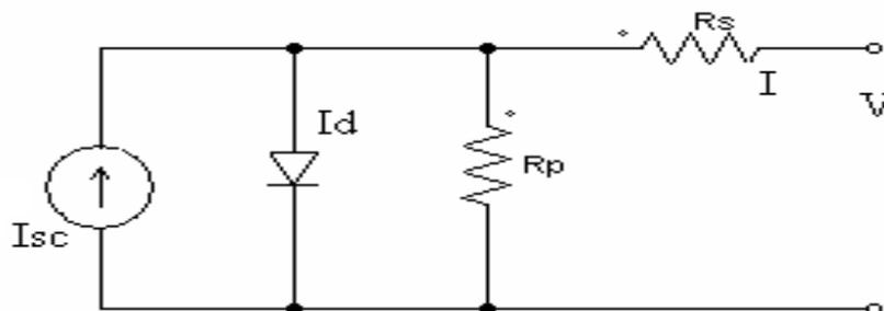
Fig. 2 Equivalent circuit of a PV module
