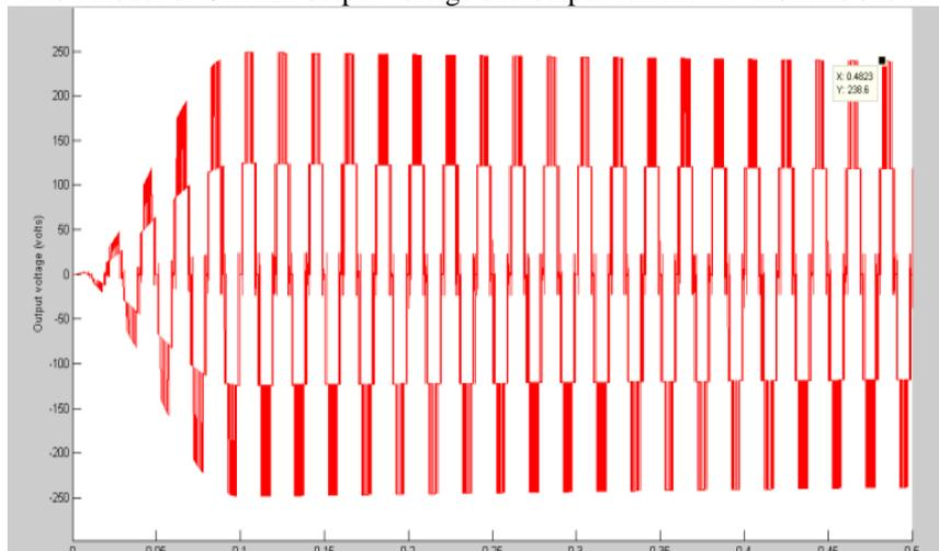
Fig. 8 Output voltage(230V) waveform for CHMLI inverter
