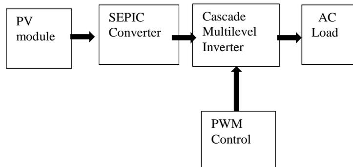
Fig.1 Overall block diagram
