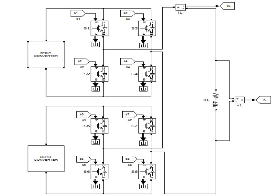
Fig. 7 SIMULINK model for SEPIC&CHMLI
