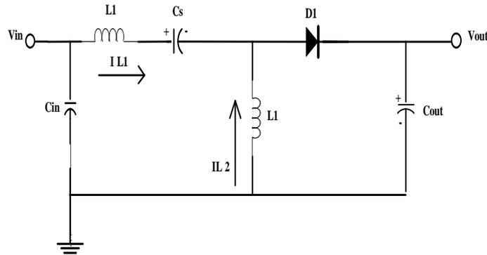
Fig.4 SEPIC Converter Current Flow
