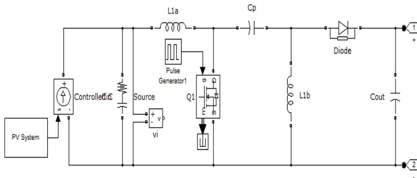
Fig.5 SIMULINK model for SEPIC converter
