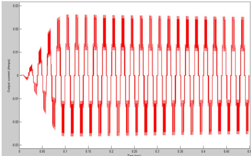
Fig. 9 Output current waveform for CHMLI inverter
