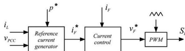
Fig.2: Inverter control scheme
