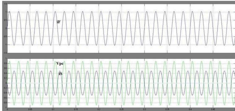
Fig. 14: Steady-state operation of 2 Kw load connected active power generation with inverter current (top), grid current vs grid voltage (bottom)
