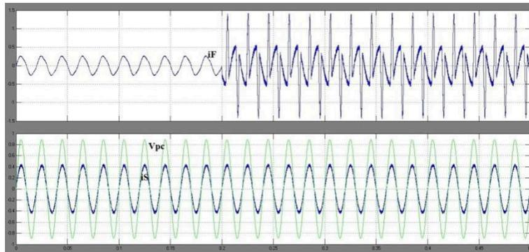
Fig. 17: Inverter transient response during non-linear load turn-on for inverter current (top), grid current vs grid voltage (bottom)
