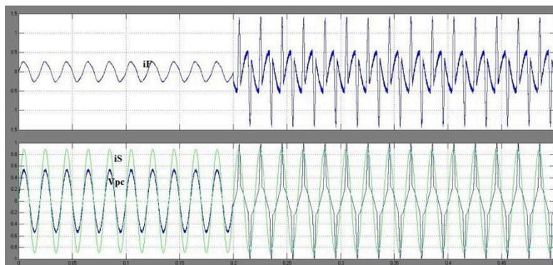
Fig. 18: Inverter transient response for non-linear load turn-on for inverter current (top), load current vs grid voltage (bottom)
