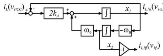
Fig.4: SSI filter applied for the load current and for the PCC voltage
