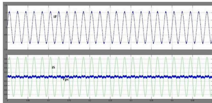
Fig. 12: steady-state operation of the inverter injecting the active power by resistive load of 2 Kw
