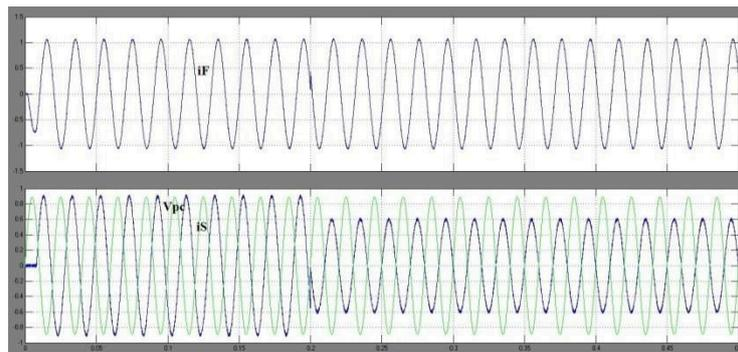
Fig. 22: Inverter transient response for step reactive power compensation when the injected active power is 3 Kw inverter current (top), grid current vs grid voltage (bottom)
