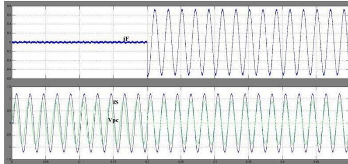
Fig. 20: Inverter transient response when only reactive power compensation is enabled and load is resistive, inverter current (top), grid current vs grid voltage (bottom)
