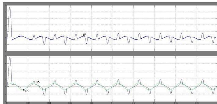
Fig. 16: State operation of the inverter injecting 1kw active power and compensating the current harmonics of the load.
