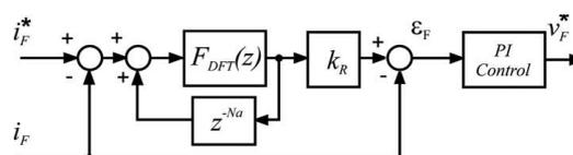
Fig.7: Current control scheme
