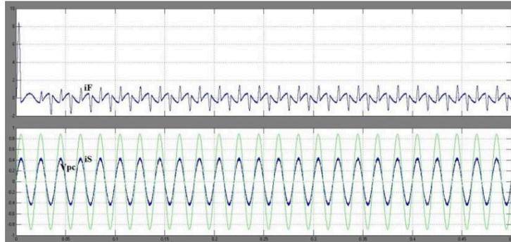
Fig. 17: Steady state operation of inverter injecting 1 Kw active power and compensating harmonics of the local load for inverter current (top), grid current Vs grid voltage (bottom)
