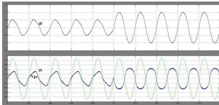
Fig. 15: Inverter transient response during a step-up of the injected active power (2Kw linear load) for inverter current (top), grid current vs grid voltage (bottom)
