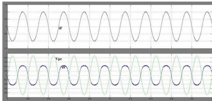
Fig. 21: Steady-state operation of 3Kw active power generation with reactive power compensation inverter current (top), grid current vs grid voltage (bottom)
