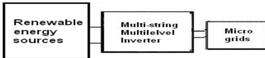
Fig.1 Block diagram of multistring multilevel inverter for microgrid application
