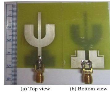
Fig 8: Picture of fabricated antenna
