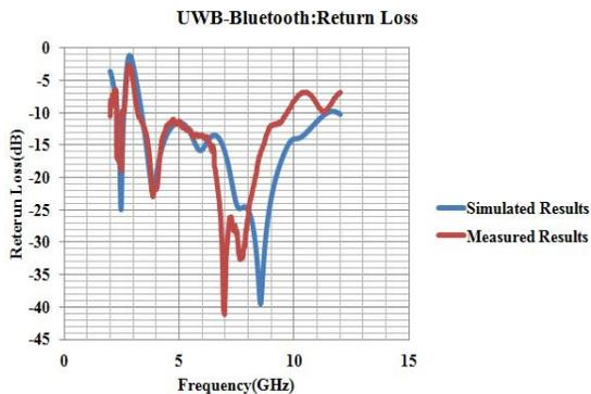
Fig 10: UWB and Bluetooth Return loss
