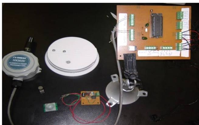
Figure 12. Final design of the prototype circuit board
