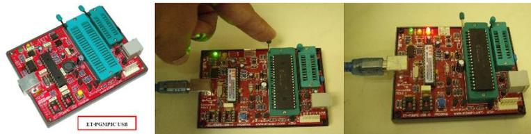
Figure 3. a) ET-PGMPIC USB Development Board (left). b) Connection of the microcontroller with the ET-PGMPIC USB Development Board (middle). c) Programming process (right).
