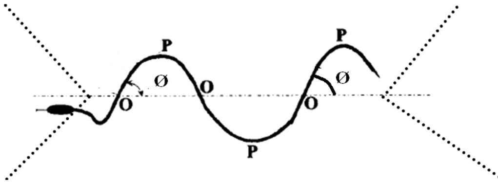
Figure 2: Path followed by the data packet in Snake Serpentine Algorithm
