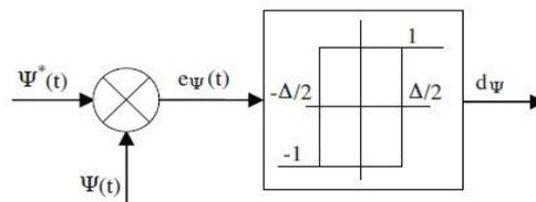
Figure 5 Two Level Hysteresis Band Control
