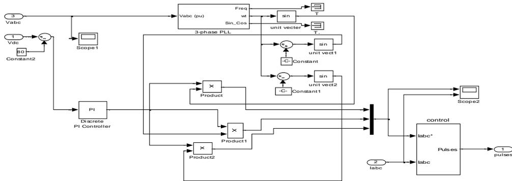
Figure 8 Control logic for pulses
