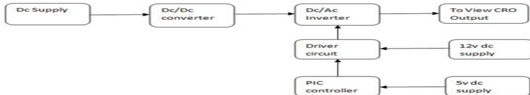
Figure 2. Block diagram of system interconnected diagram
