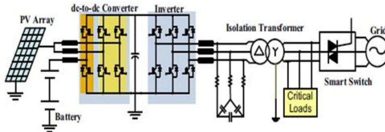
Fig 4 shows system interconnected diagram
