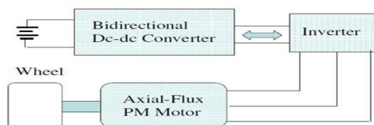
Figure 3 Bidirectional DC-DC converters in energy regenerative system
