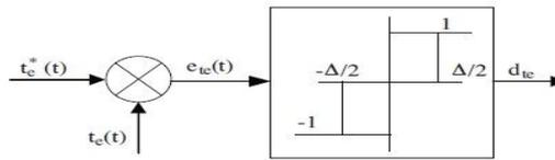
Figure 6 Three Level Hysteresis Band Control
