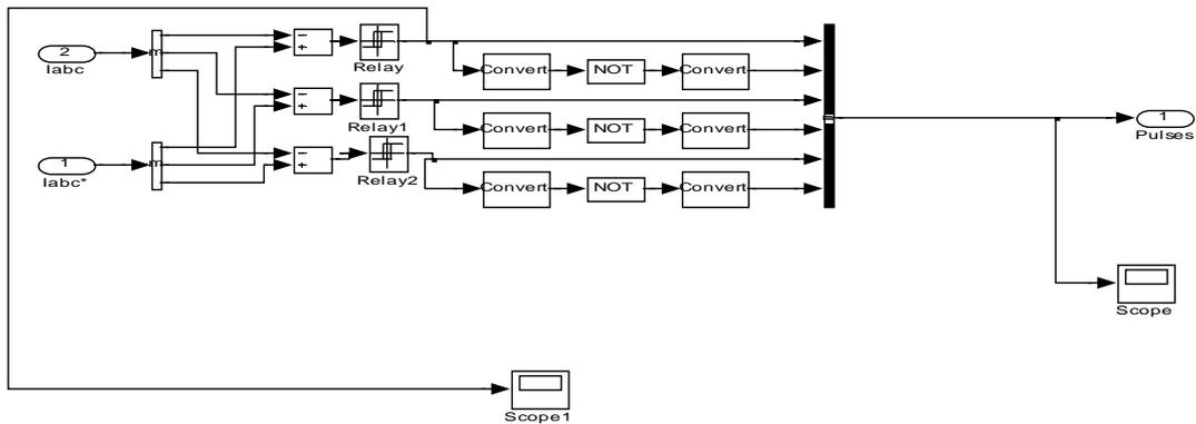
Figure 9 Hysteresis control logic block
