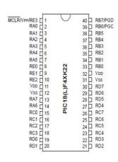
For this project we are using a 40-pin PIC18LF45K22 Microcontroller which is a PIC type Microcontroller. PIC is a family of modified Harvard architecture microcontrollers made by Microchip Technology, derived from the PIC1650 originally developed by General Instrument's Microelectronics Division. The name PIC initially referred to "Peripheral Interface Controller".
