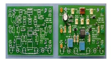
Before a PCB can be physically fabricated it has to be decide where all the components will be placed and arranged and how the PCB traces will connect the different components. This process is colled PCB design.
