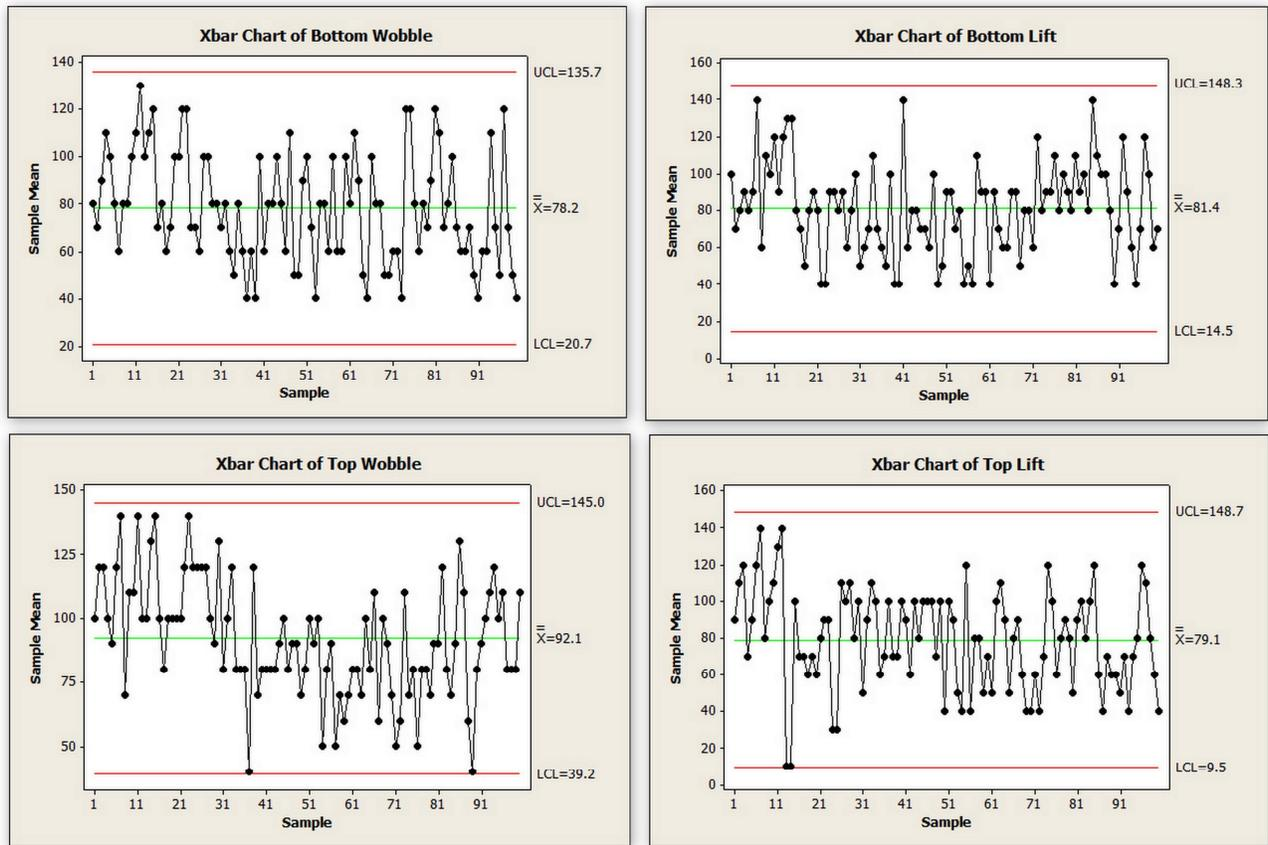
Figure 3 X-bar Chart for Bottom Wobble, Bottom Lift, Top Wobble and Top Lift
