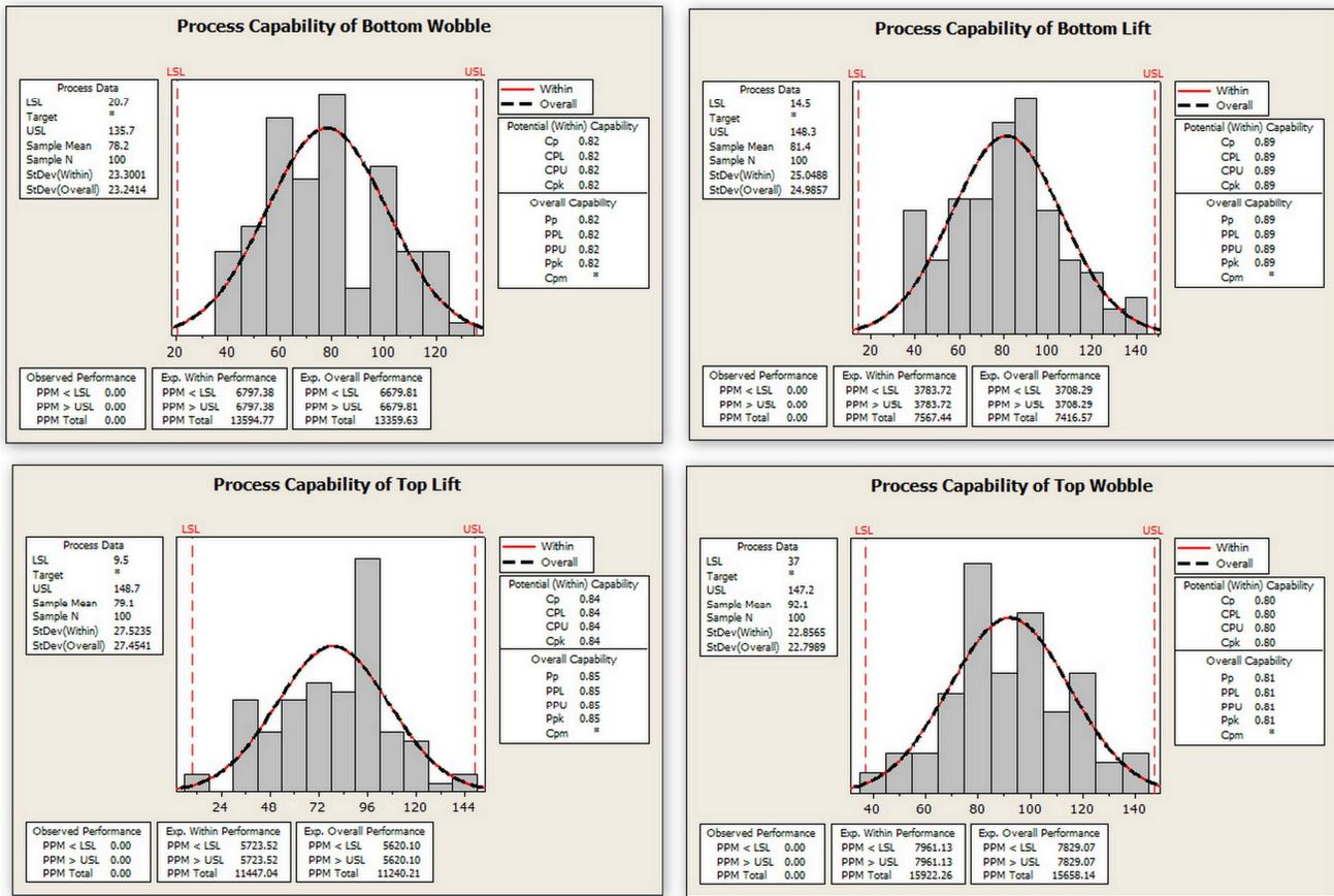
Figure 7 Process Capability for Bottom Wobble, Bottom Lift, Top Wobble and Top Lift
