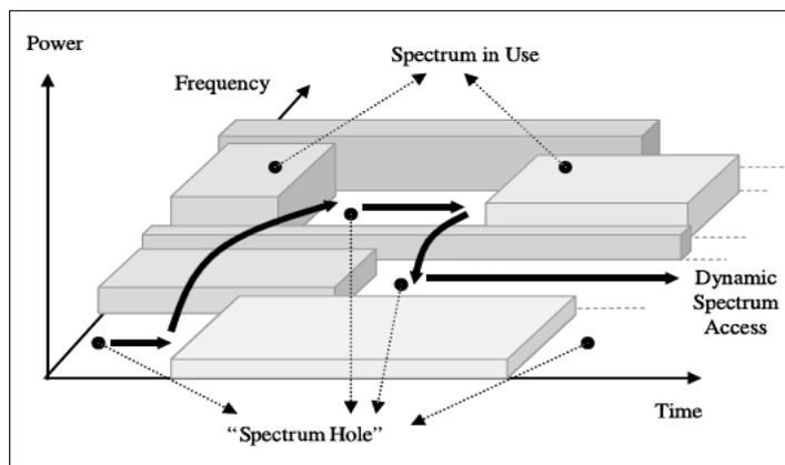
Fig.1 Concept of spectrum hole.
