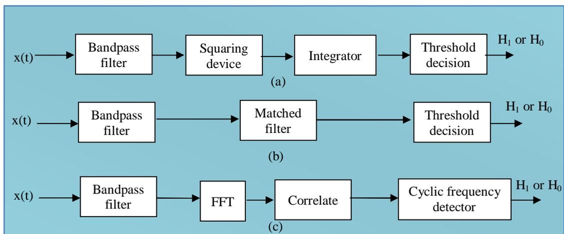
Fig 1: Block diagrams for narrowband spectrum sensing techniques: a) energy detection; b) matched filtering; c) cyclostationary feature detection
