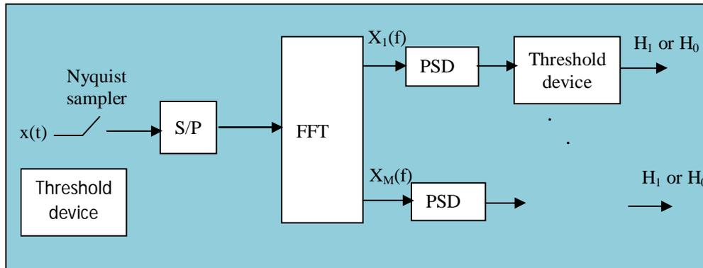
Fig 2: block diagram of Nyquist wideband spectrum sensing techniques
