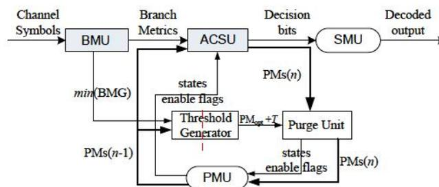
Fig.5. VD with two-step pre-computation T-algorithm
