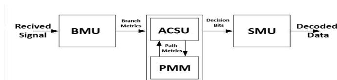
Fig.1. Viterbi decoder functional diagram.
