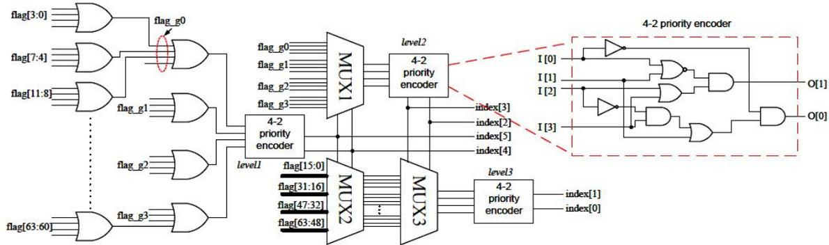
Fig.6. Architecture of 64-to-6 priority encoder
