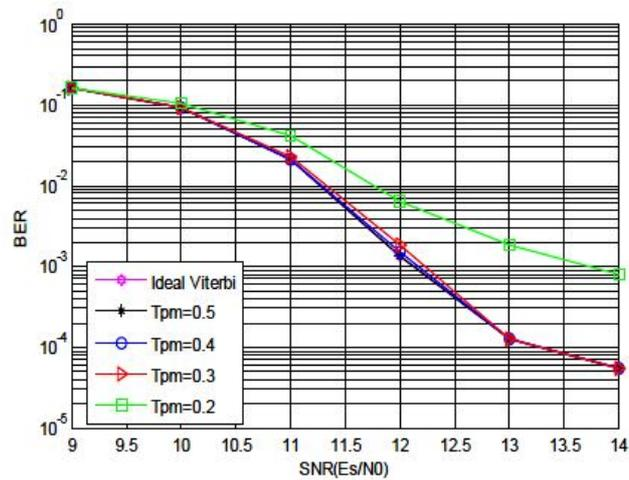
Fig.4. BER Performance of T-algorithm
