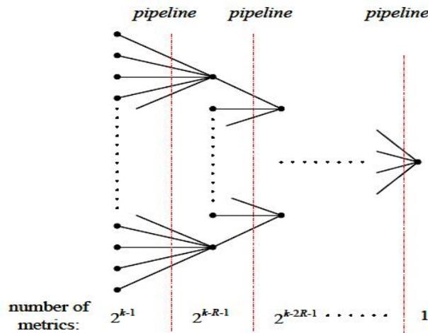
Fig. 2. Topology of pre-computation pipelining
