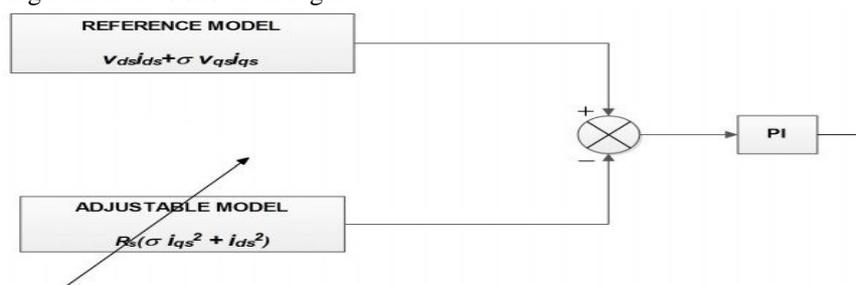
Fig.2.MRAC based stator resistance estimation technique
