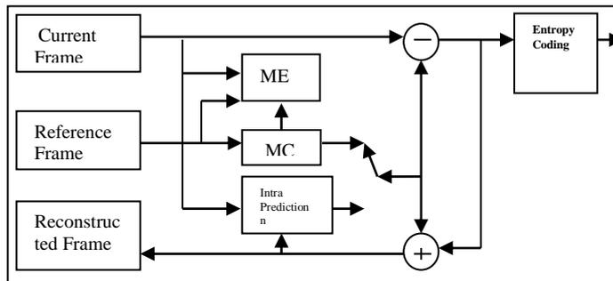
Figure 2: Proposed motion estimation and codec process flow.
