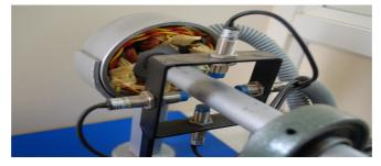
Fig.6. Rotor sensor arrangement to sense the rotor position.
