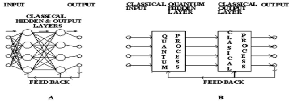
Figure 1. (A) Classical and (B) Hybrid Quantum Neural Network Learning by Feed Back
