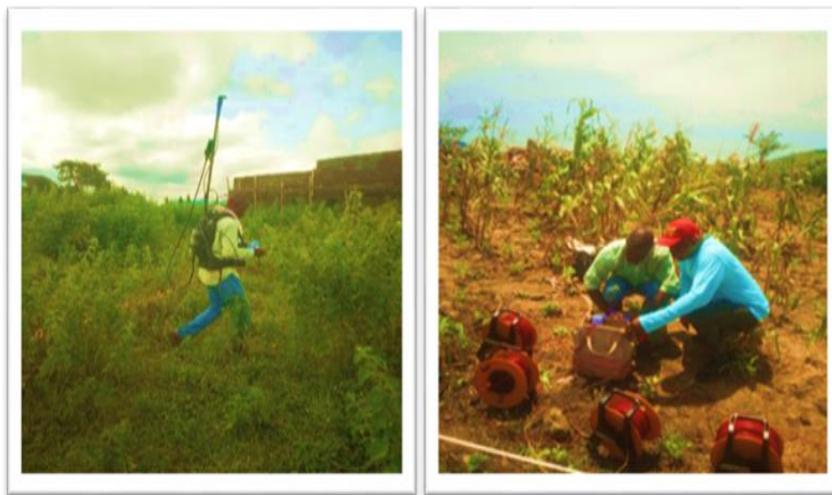
Figure 4. Magnetic and geo-electrical data acquisition.
