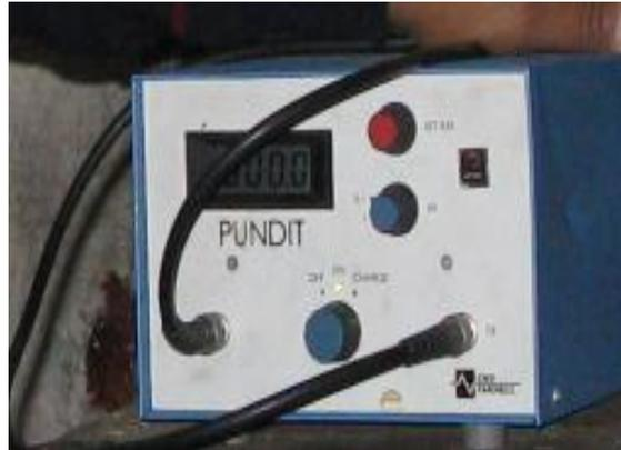
Fig.3. Portable Ultrasound Non destructive Digital Indicator Tester Equipment (PUNDIT)
