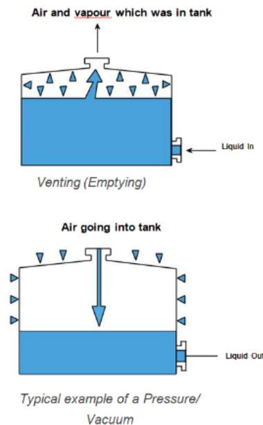
**Figure 2.** Dome roof tanks.
