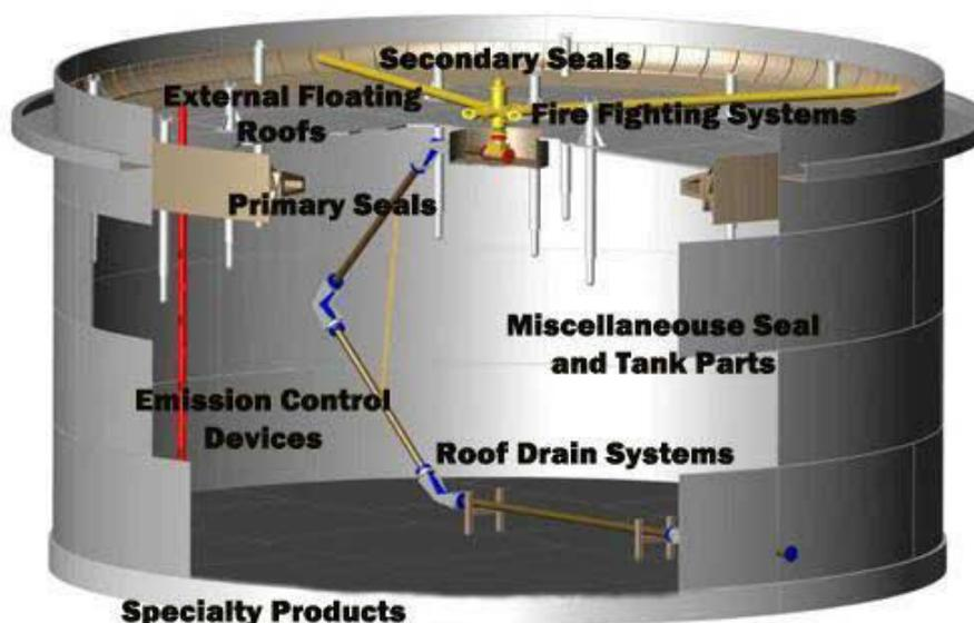
Figure 4. External floating roof tank.
