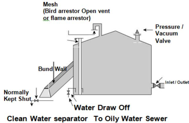
**Figure 1.** Fixed roof tank.
