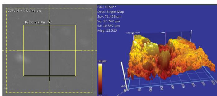
Figure 9. The optical profile of the W2.5%Lig sample after heat treatment at 100 °C
