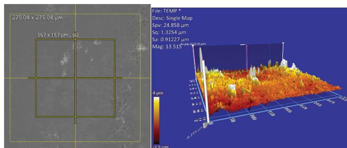
Figure 7. The optical profile of the W5%Lig sample after heat treatment at 100 °C
