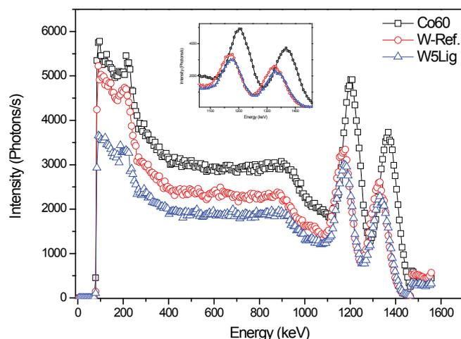
Figure 10. The comparative spectrums of the attenuation of gamma radiation between Co-60, standard tungsten, and W5%Lig sintered at 90 °C
