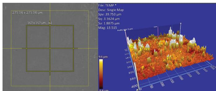
Figure 6. The optical profile of the W5%Lig sample after heat treatment at 90 °C
