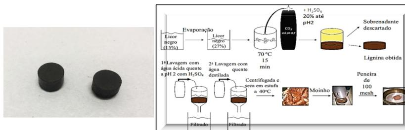
Figure 2. Shows the samples of W2.5%Lig and W5%Lig after pressing
