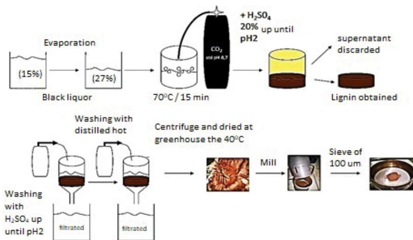
Figure 1. Experimental scheme of the kraft lignin
