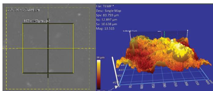
Figure 8. The optical profile of the W2.5%Lig sample after heat treatment at 90 °C
