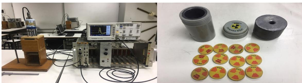
Figure 5. a) Experimental scheme measuring gamma radiation; b) Source cobalt (Co-60)
