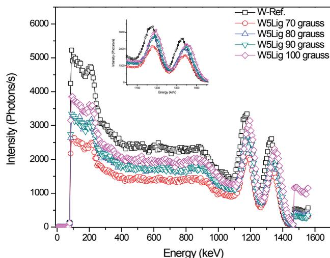
Figure 11. The comparative spectrums of the attenuation of gamma radiation between standard tungsten and the W5%Lig composite sintered at 70, 80, 90, and 100 °C
