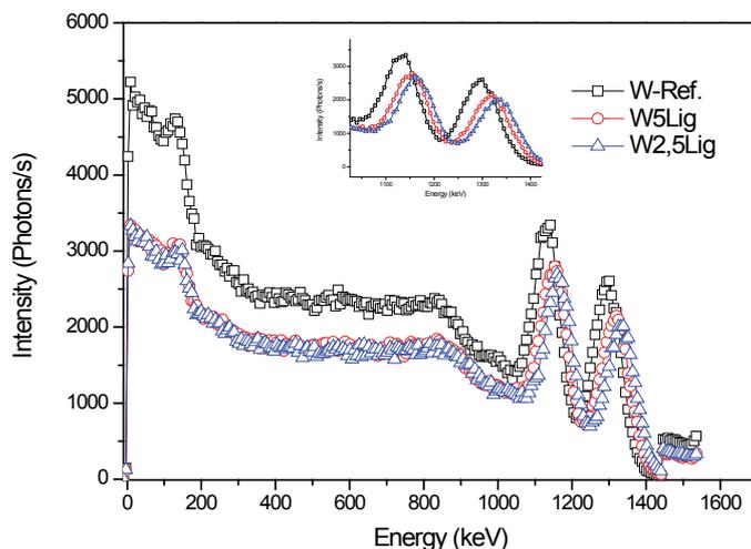
**Figure 12.** The comparative spectrums of the attenuation of gamma radiation between standard tungsten and the W5%Lig and W2.5%Lig composites sintered at 90°C
