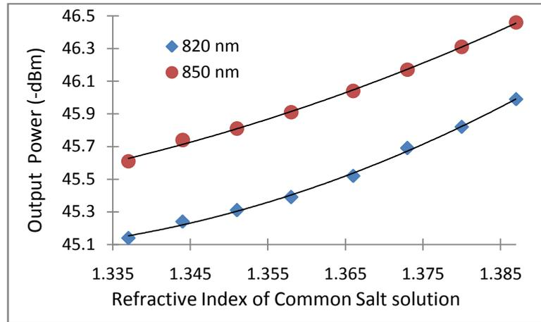
Fig.3. Graph showing variation of output power with refractive index of guiding liquid common salt solution at operating wavelengths 820nm & 850nm
