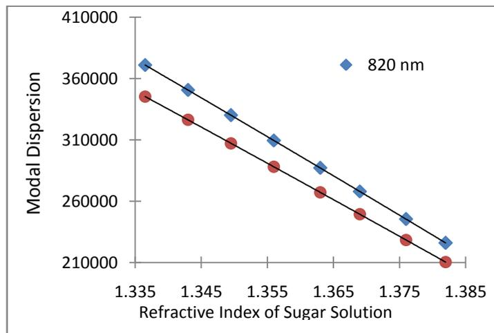
Fig(10):The relation showing variation of Modal Dispersion with refractive index at operating wavelengths 820nm and 850nm for guiding liquid of sugar solution.
