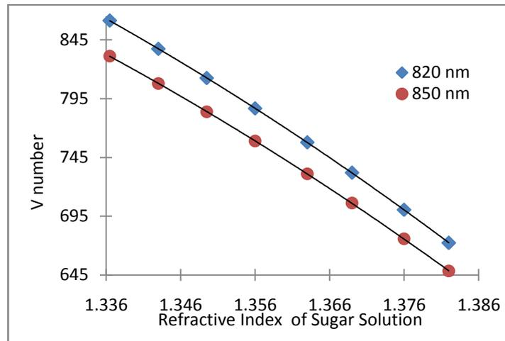
Fig(8):The relation showing variation of V-number with refractive index atoperating wavelengths 820nm and 850nm for guiding liquid of sugar solution
