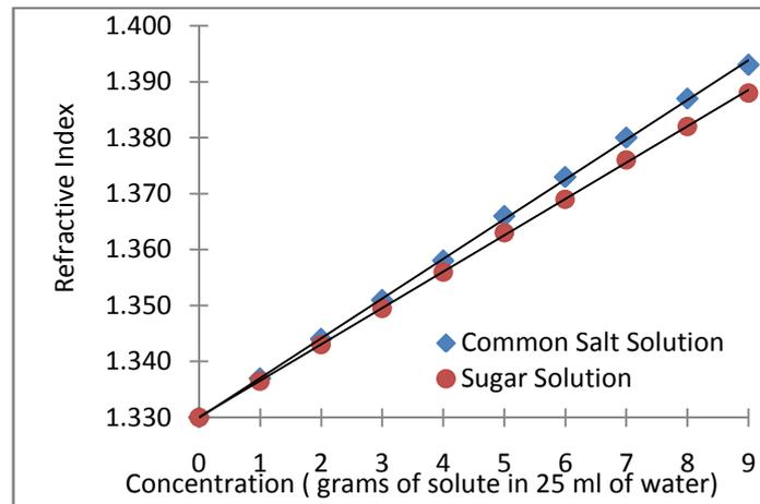
Fig (1): Graph indicating the relation between concentration and refractive index of common salt solution and sugar solutions
