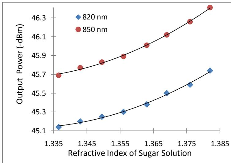
Fig(4): Graph showing the relationship between refractive index and output power at operating wavelengths 820nm and 850nm for guiding liquid of Sugar solution
