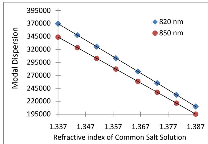
Fig(9):The relation showing variation of Modal Dispersion with refractive index at operating wavelengths 820nm and 850nm for guiding liquid of common salt solution
