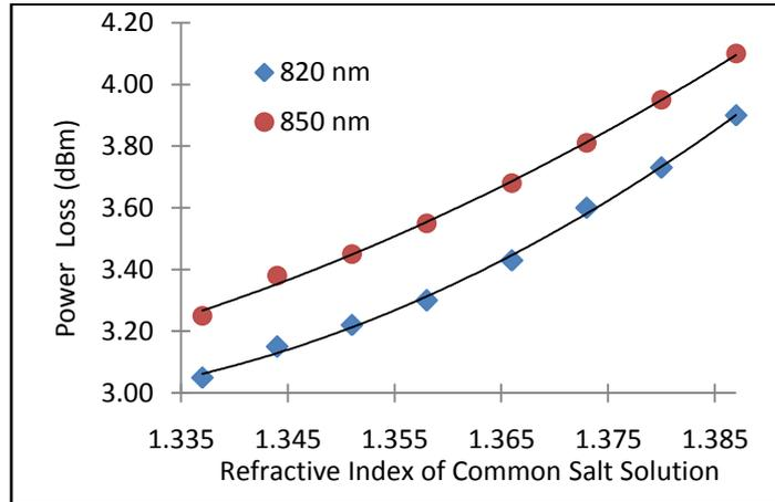
Fig(5): Graph showing the relationship between refractive index and power loss at operating wavelengths 820nm and 850nm for guiding liquid of common salt solution
