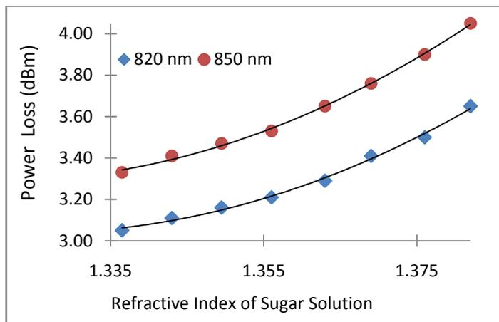
Fig(6): Graph showing the relationship between refractive index and power loss at operating wavelengths 820nm and 850nm for guiding liquid of sugar solution
