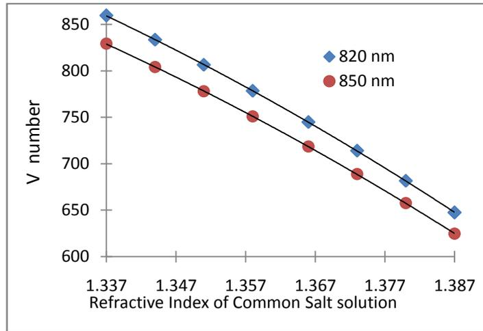
Fig(7):The relation showing variation of V-number with refractive index at operating wavelengths 820nm and 850nm for guiding liquid of common salt solution
