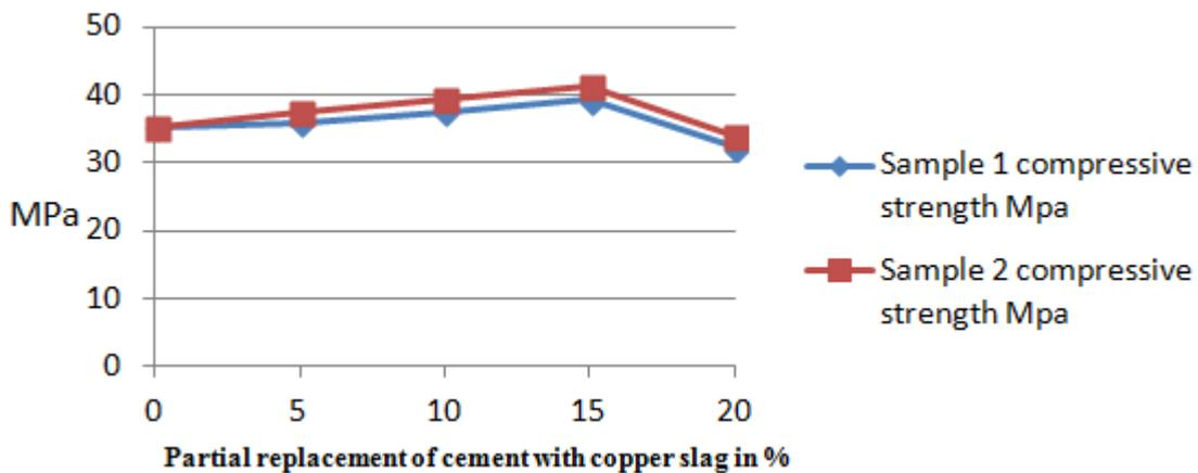
Fig.2. Comparison of Compressive Strengths of M30 mix design
