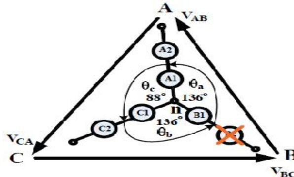
Fig no.5 The “neutral shift method for reconfiguration technique
