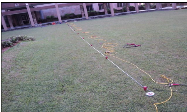
2(c): Geophones in a linear array
