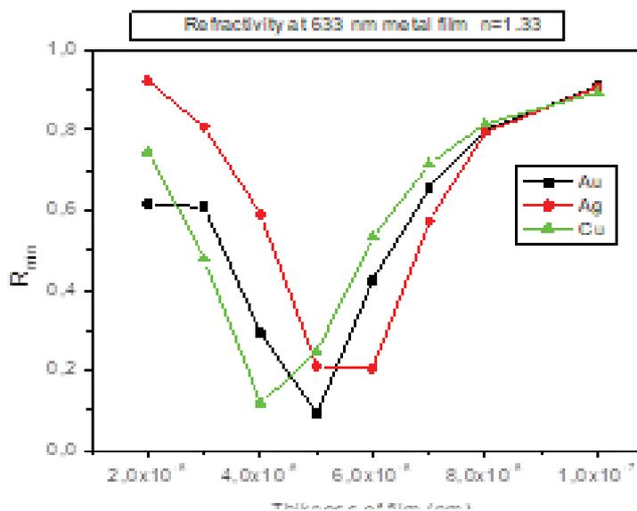
**Figure 5.**  $R_{min}$  of Au, Ag and Cu films in water, as a function of the thickness of the metal.
