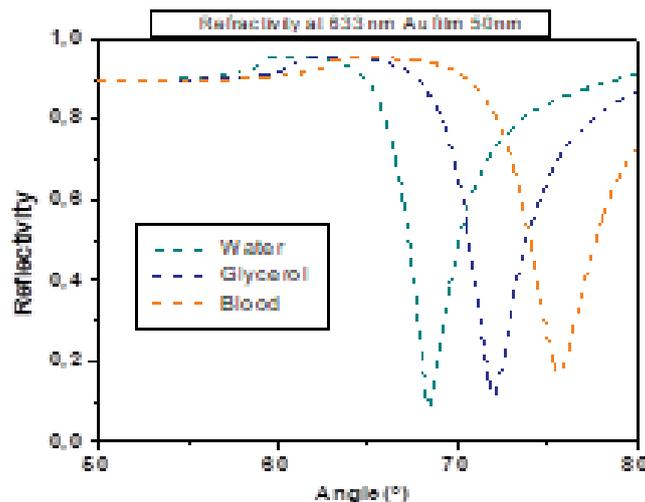
**Figure 4.** Reflection spectra of a 50 nm **thick** Au film in: water ( $n=1.33$ ), glycerol ( $n=1.357$ ), blood ( $n=1.38$ ).
