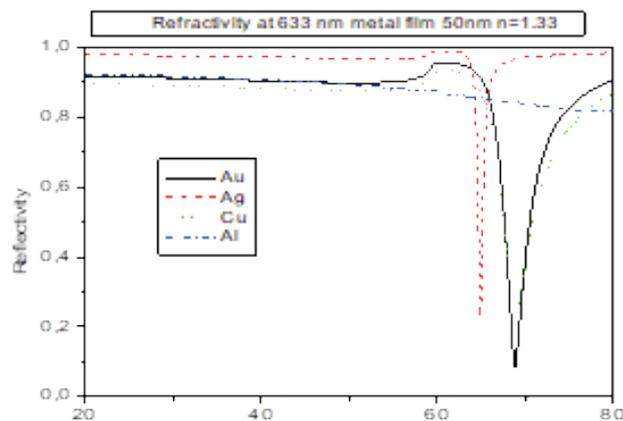
**Figure 3.** Reflection spectra of 50 nm thick Au, Ag, Cu and Al films in water.
