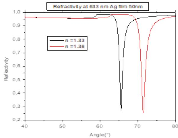
**Figure 2.** Reflection spectra of a 50 nm thick Ag film in different surrounding media:  $n=1.33$ ,  $n=1.38$ .
