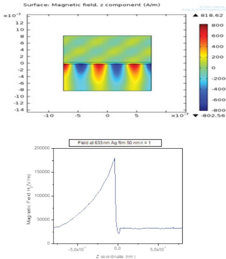
**Figure 6.** Hz magnetic field profile of a 50 nm thick Ag film in air.
