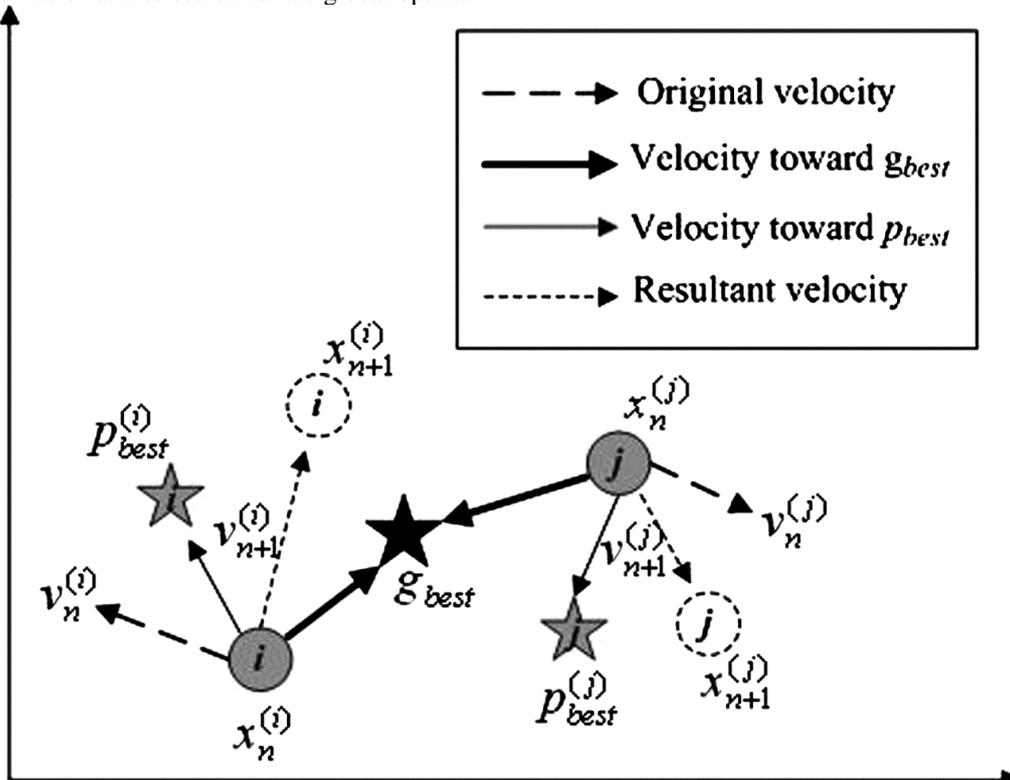
Fig 3: Particle Swarm optimization Technique
