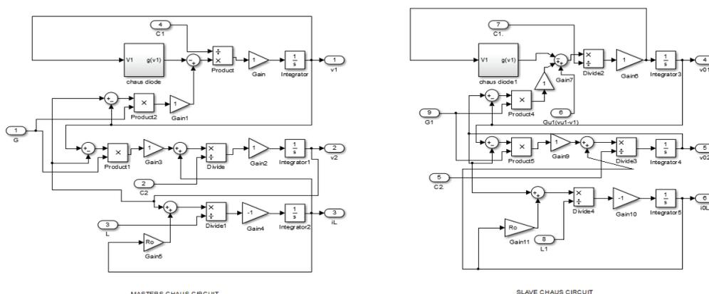
Figure 6. Model for master and slave Chua's oscillator.
