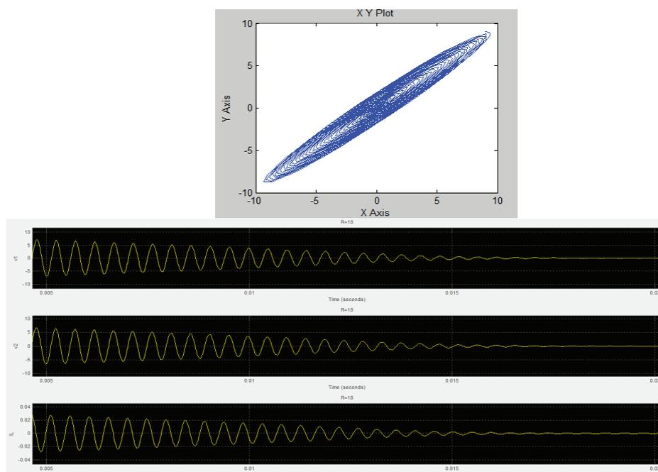
Figure 10. Transient waveform (a): phase trajectory; (b): when  $R_1 = 18\Omega$ .
