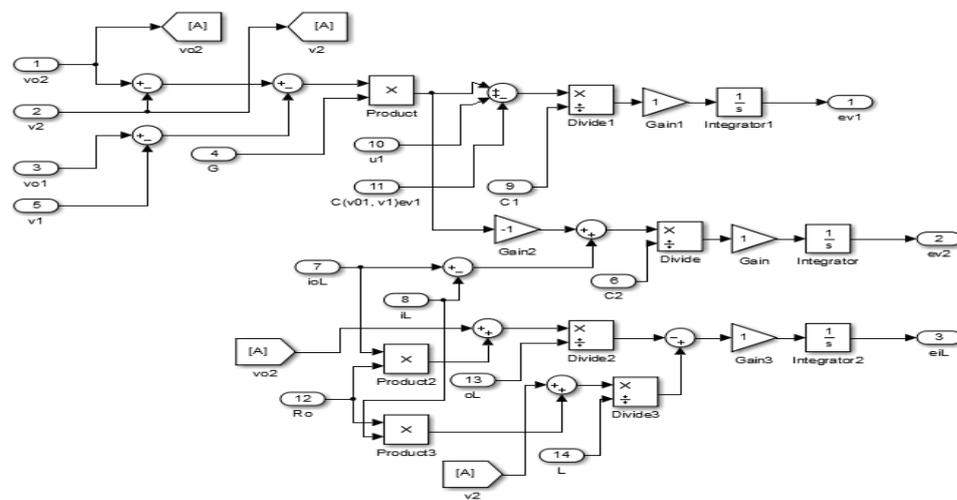
Figure 7. Model for master/slave Chua's oscillator.
