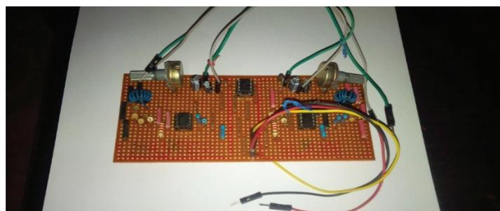
Figure 8. The Chua circuit implementation of the design.
