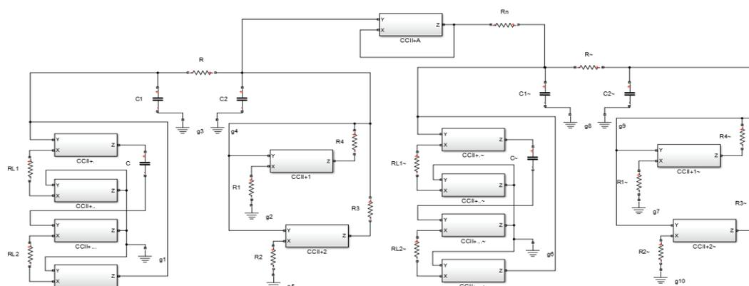
Figure 4. Current conveyors based realization of two Chua's oscillator.
