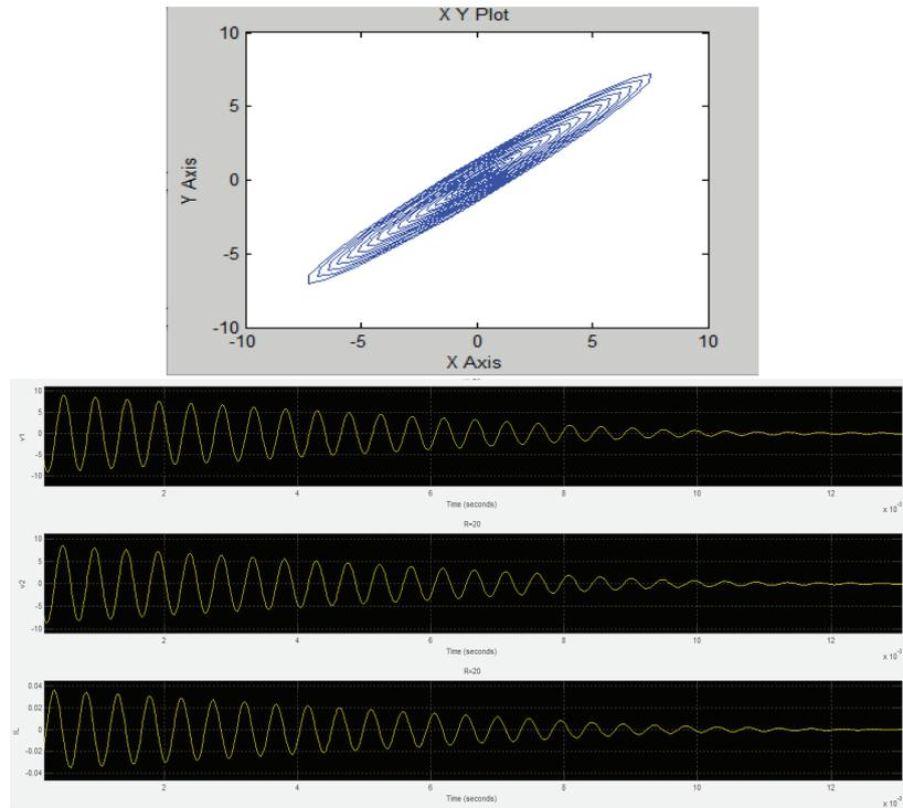
**Figure 13.** Transient waveform 4 (a): phase 4 space trajectory; (b): when  $R_2=20\Omega$ .
