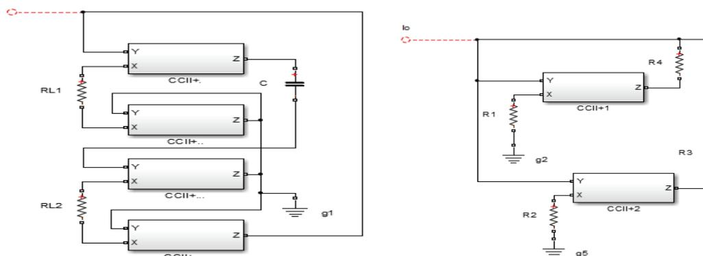
Figure 1. (a): simulated inductance in CCII+; (b): chua's diode in CCII+.
