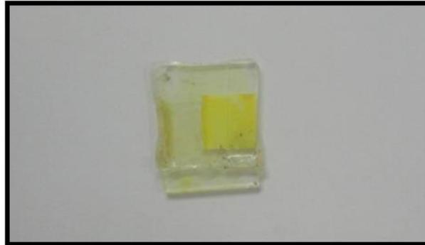
**Figure 2:** Actual photographs of  $\text{In}_2\text{S}_3$  films deposited on  $\text{TiO}_2$  by CBD method in alkaline bath on FTO-coated glass substrates.
