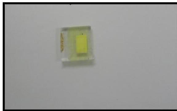
Figure 1: Actual photographs of In<sub>2</sub>S<sub>3</sub> films deposited on TiO<sub>2</sub> by CBD method in acidic bath on FTO-coated glass substrates.
