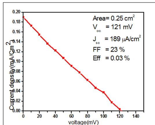
**Figure 5: Photo-current density-photovoltage (J-V) characteristics of SSSC based on FTO  $\text{TiO}_2 / \text{In}_2\text{Se}_3 / \text{Pt}$ - (acidic bath).**
