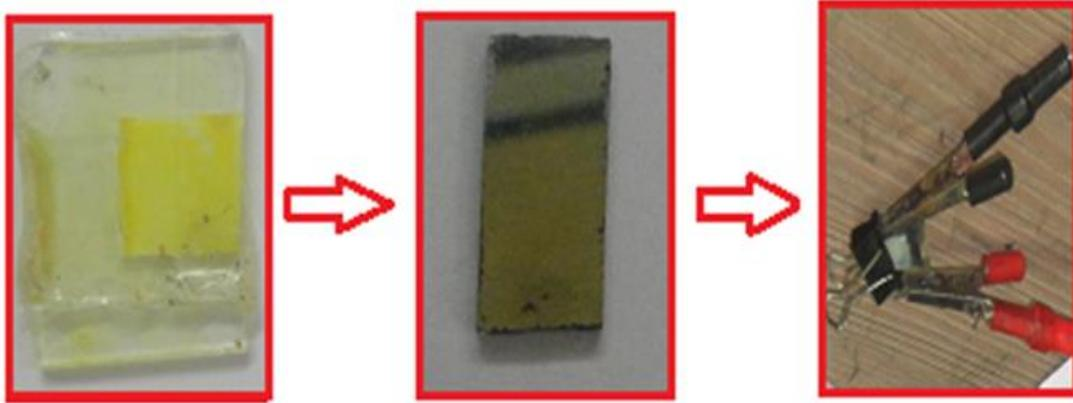
**Figure 4: Actual photographs of depositing  $\text{In}_2\text{S}_3$  on  $\text{TiO}_2$  in alkaline bath on FTO-coated glass substrates and fabricating it for SSSC.**
