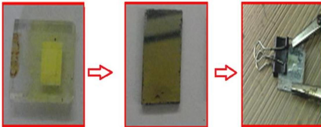
**Figure 3:** Actual photographs of depositing  $\text{In}_2\text{S}_3$  on  $\text{TiO}_2$  in acidic bath on FTO-coated glass substrates and fabricating it for SSSC.
