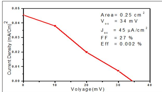
**Figure 6: Photo-current density- photovoltage (J-V) characteristics of SSSC based on FTO TiO<sub>2</sub> / In<sub>2</sub>Se<sub>3</sub>/ Pt- (alkaline bath).**
