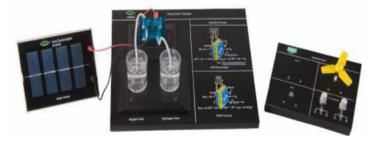
Fig. 6: Solar-hydrogen fuel cell hardware system
