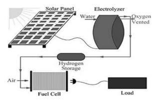
Fig. 3: Fuel cell based electricity generation
