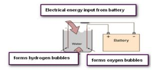
Fig. 4: Electrolysis process of water
