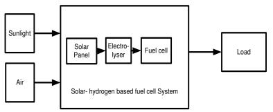
Fig. 5: Experimental setup for solar-hydrogen based fuel cell system
