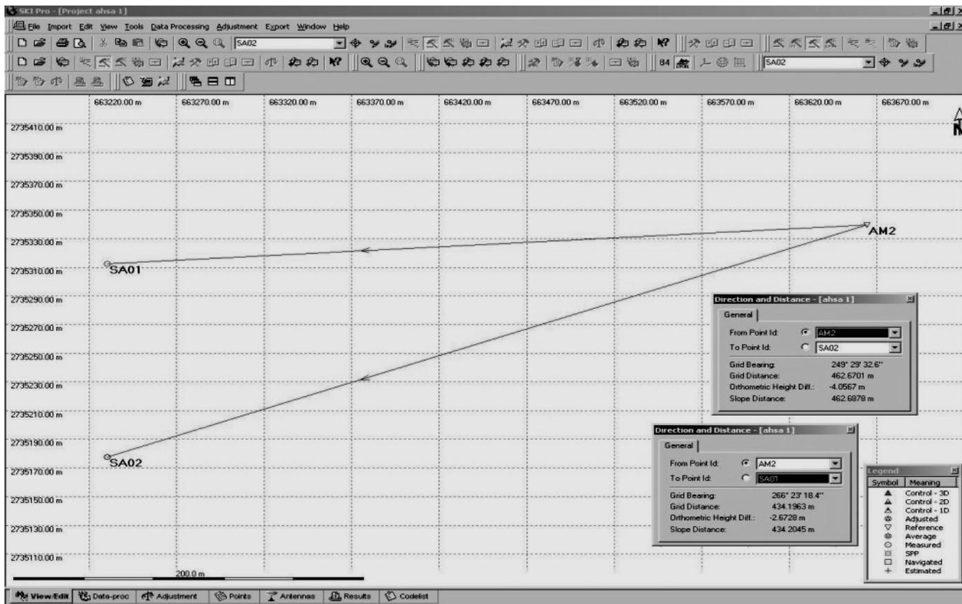
Figure 8. Direction and distance of SA01 and SA02 link to control AM2.
