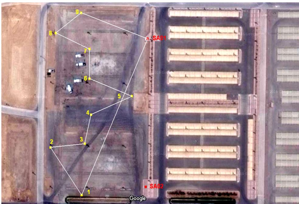
Figure 4. Traverse reference test network.
