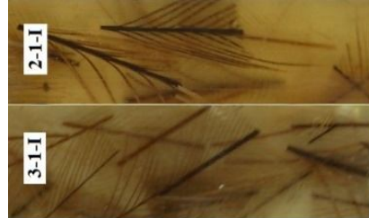
Fig. 1 Sample Specimens of 'Emu' feather fiber epoxy composites
