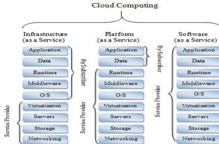
Figure3: Service Model of Cloud Computing
