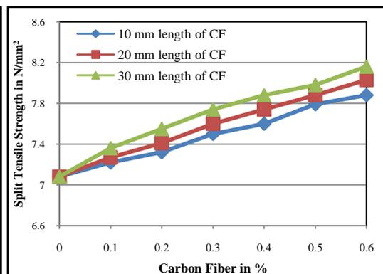
Fig.2. Split Tensile Strength V/s carbon fiber
