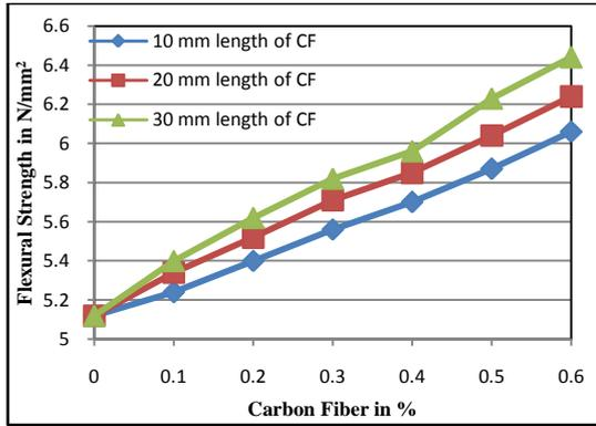
Fig.3. Flexural Strength V/s carbon fiber
