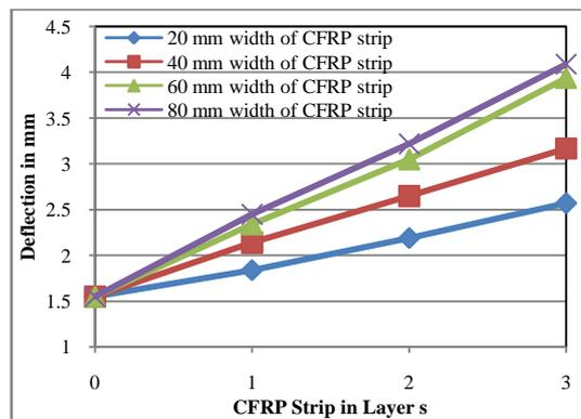
Fig.7. Load deflection response (for CFRP beam).
