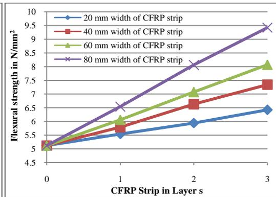
Fig. 6 Flexural Strength (for CFRP beam).
