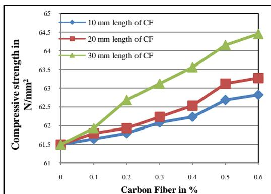
Fig.1. Compressive Strength V/s carbon fiber
