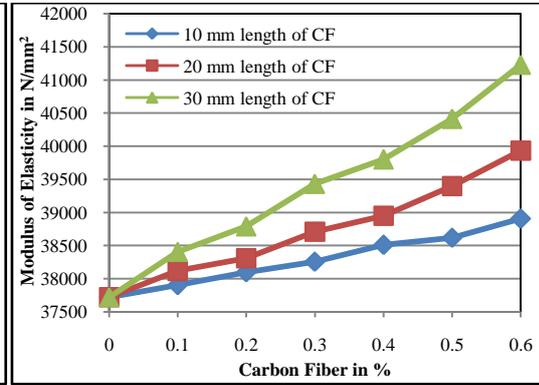
Fig.4. Modulus of Elasticity V/s carbon fiber
