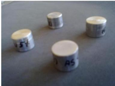
**Fig 3.5:** Hardness test specimens
